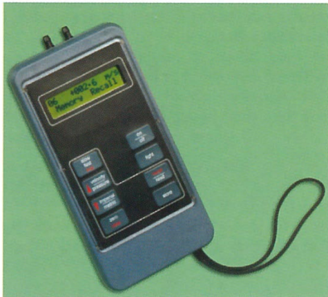
Figure 7.8 Volume flow indicating instrument
